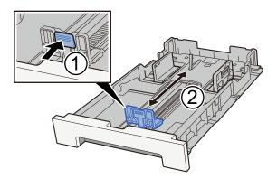
2 Adjust the paper length guides to the paper size required. Press the paper length adjusting tab and slide the guides to the paper size required. (Cassette 1 only)
