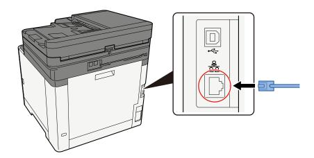
**2** Connect the other end of the cable to the hub.
