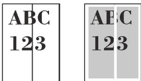
Laser scanner cleaning needs to be performed.
