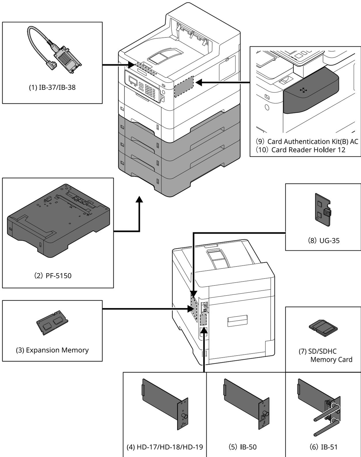
1 IB-37/IB-38 <Wireless network interface (USB: 5GHz/2.4GHz)>
