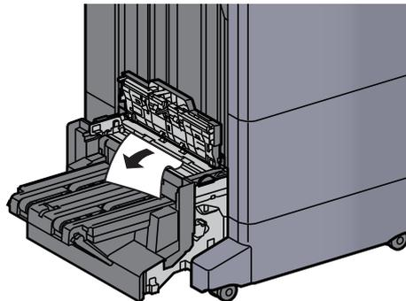
**14** Open the folding unit conveyor guide.
