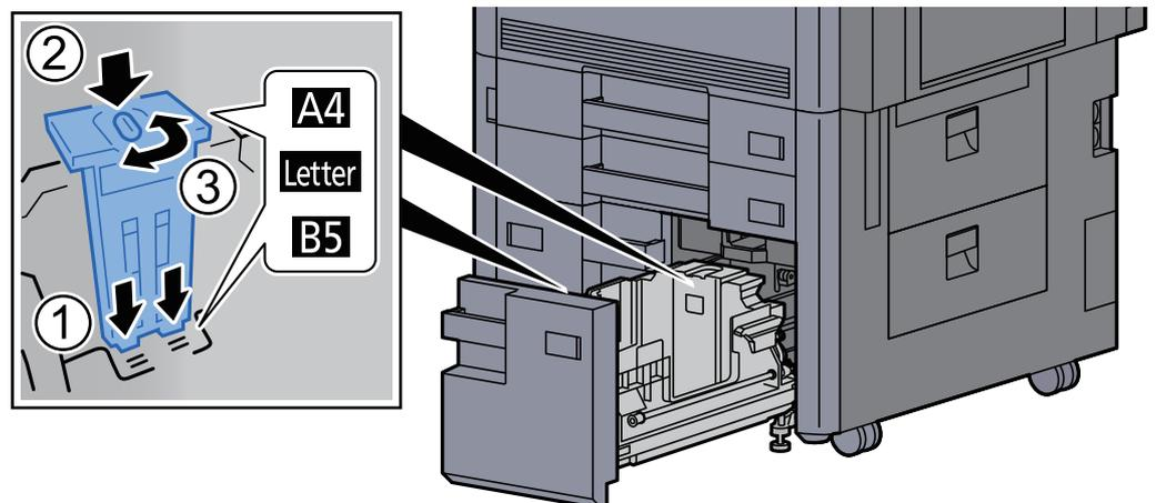
Make sure that the top of the Paper Size Guide (A) matches the paper size to be used, attach the clamp, and rotate the clamp to lock it.
