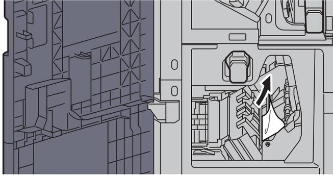
**3 Remove the Staple Cartridge Holder (B) or (C).**
