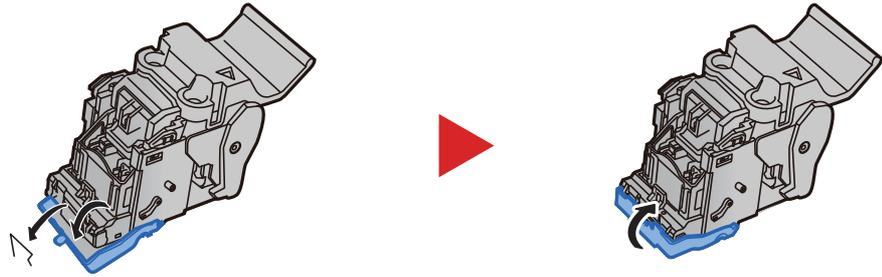
**5 Install the Staple Cartridge Holder (B) or (C).**
