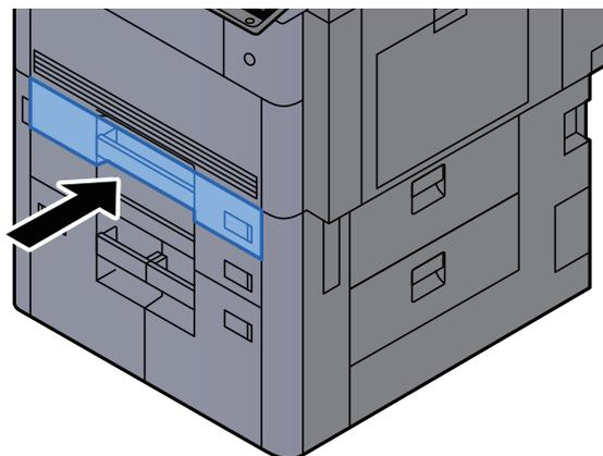
**9 For Cassette 1 and 2, insert a sheet of the required paper size and type, as shown in the illustration.**
