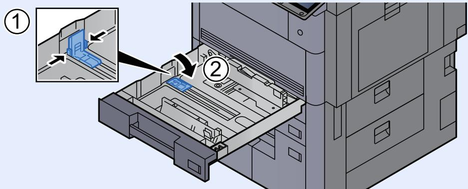
**3 Press the paper width guide lock to release the lock.**
