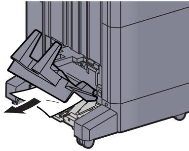
**9 Press the release lever to pull the folding unit out.**
