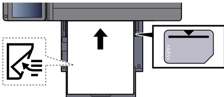
Insert the paper along the paper width guides into the tray until it stops.
