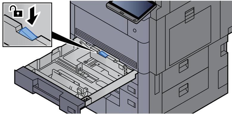
**4 Adjust the position of the paper width guides located on the left and right sides of the cassette.**
