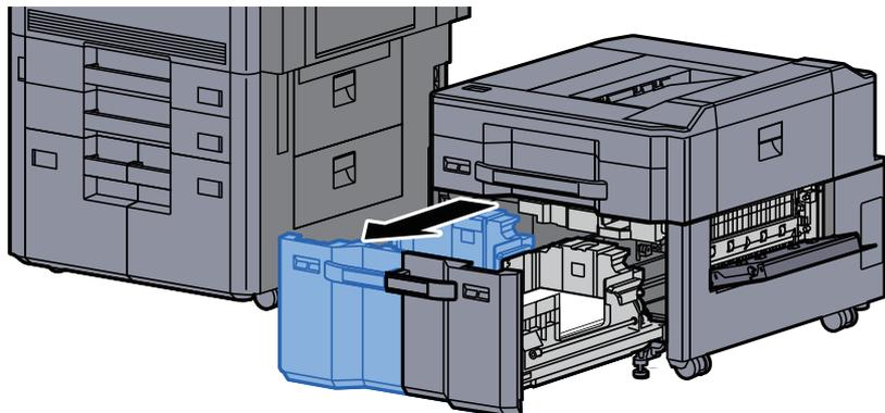
**7 Pull out side feeder paper feed unit (B1).**
