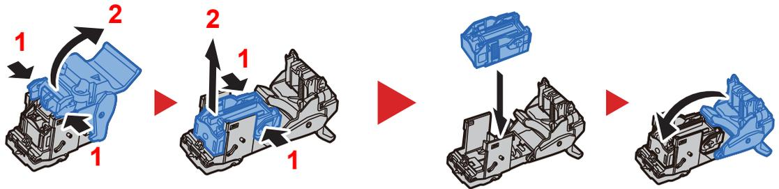
**4 Install the Staple Cartridge Holder (B) or (C).**
