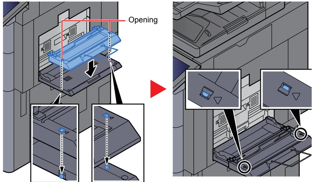
Fit the openings on the sides of the banner tray onto the tabs on the sides of the multipurpose tray, and press into place.
