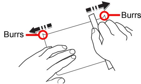
Before loading Hagaki (Cardstock) into the MP tray, fan them and align the edges. If the Hagaki (Cardstock) paper is curled, straighten it before loading. Printing onto curled Hagaki (Cardstock) may cause jams.
