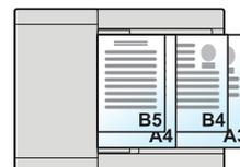
\* Set the originals of A4 and B5 with vertical orientation.
