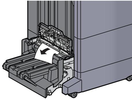
**11** Open the folding unit conveyor guide.
