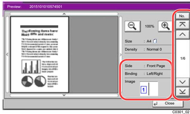
When printing duplex, it is possible to switch between the front side and the reverse side.
