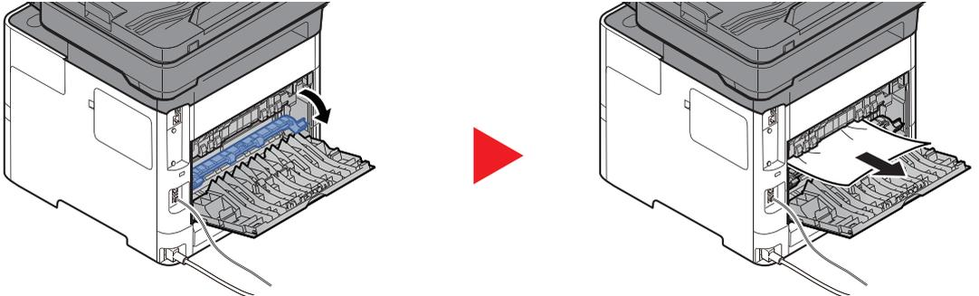
If you cannot find a paper jam, try checking inside the rear of the machine.
