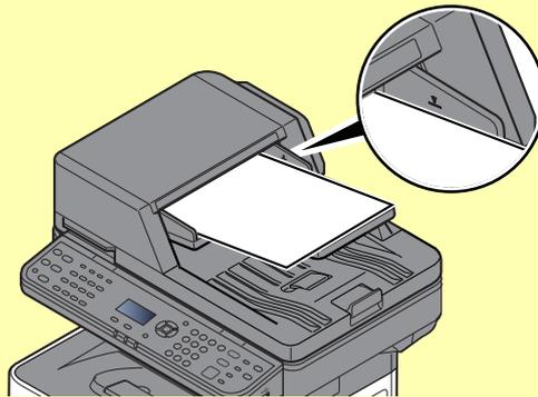
Ensure that loaded originals do not exceed the level indicator. Exceeding the maximum level may cause the originals to jam.
