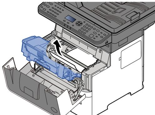
If the jammed paper appears to be pinched by rollers, pull it along the normal running direction of the paper.
