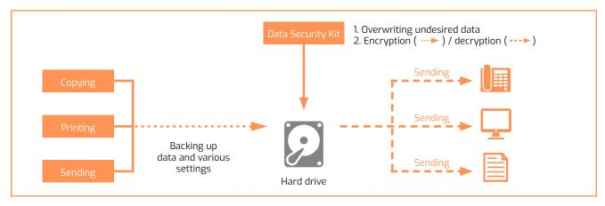
The Data Security Kit ensures the protection of your confidential information, right at the system level: it overwrites and encrypts copying, scanning and printing data, even before they are saved to the hard drive. In addition, the memory area for the output data is automatically deleted so that the data cannot be restored.
