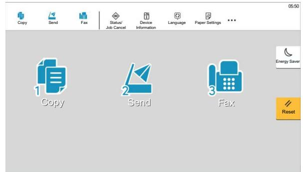
You can also control the screen using the numeric key corresponding to the number in circle. (Example: Select the [2] key on the numeric key pad to display the Send screen.)
