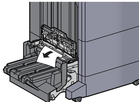
**11** Open the folding unit conveyor guide.
