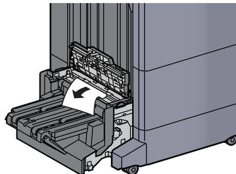
**14** Open the folding unit conveyor guide.
