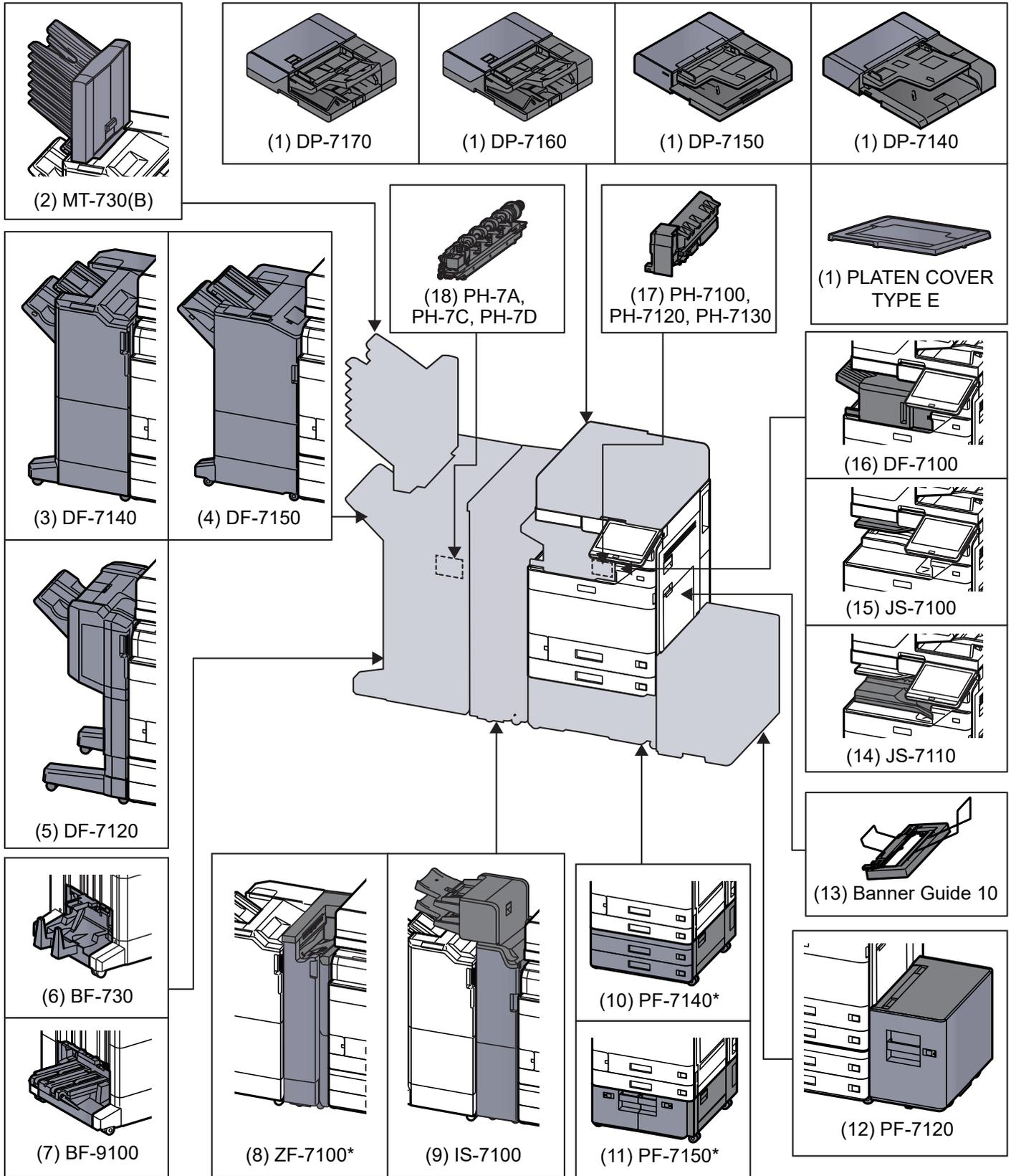
\* If the following option is installed, toppling prevention kit must be installed: PF-7140, PF-7150, PF-7120
