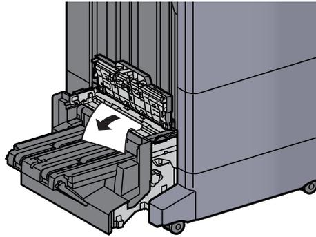
**5 Open the folding unit conveyor guide.**
