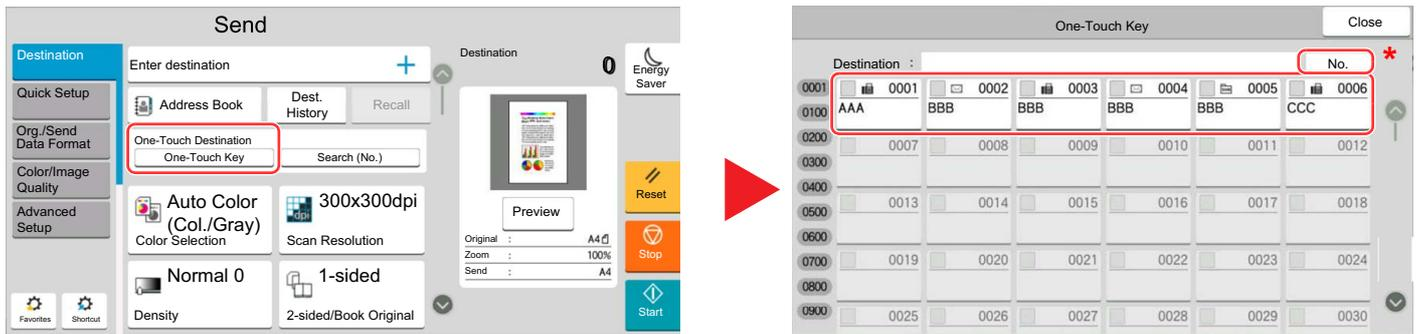
\* The [No.] key has the same function as [Search (No.)] displayed on the touch panel. Use to directly enter a number with the numeric keys, such as specifying a transmission address using a one-touch key number, or calling up a stored program using the program number. For information on one-touch key numbers, refer to the following:
