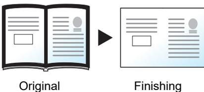
Erases black borders around the edges and in the middle of the original such as a thick book. You can specify the widths individually to erase the borders around the edges and in the center of the book.
