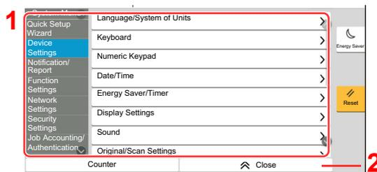
1 Displays the System Menu items. Items that are not displayed can be displayed by swiping the screen up and down.
