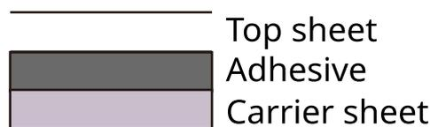
Labels consist of three layers as shown in the illustration. The adhesive layer contains materials that are easily affected by the force applied in the machine. The carrier sheet bears the top sheet until the label is used. This composition of labels may cause more problems.
