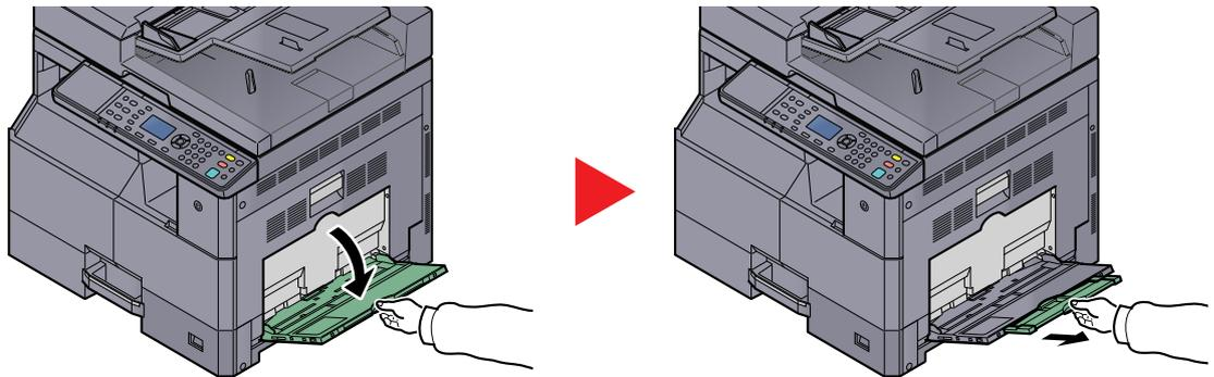
Pull out the MP tray extension to match the paper size. Refer to the label which sealed inside the machine when opening the MP tray.
