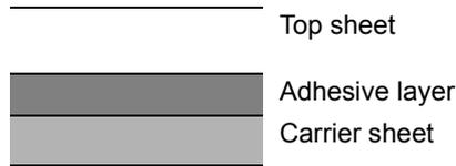
Labels consist of three layers as shown in the illustration. The adhesive layer contains materials that are easily affected by the force applied in the machine. The carrier sheet bears the top sheet until the label is used. This composition of labels may cause more problems.
