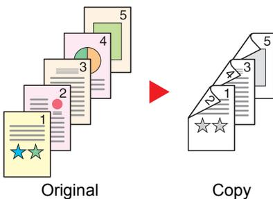
Produces two-sided copies from one-sided originals. In case of an odd number of originals, the back side of the last copy will be blank. The optional duplex unit is required.
