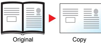
Erases black borders around the edges and in the middle of the original such as a thick book. You can specify the widths individually to erase the borders around the edges and in the center of the book.
