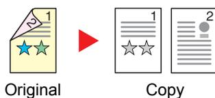
Copies each side of a two-sided original onto two individual sheets. The optional document processor is required.
