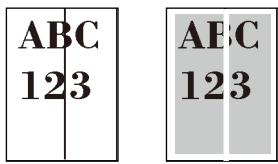
**Laser scanner cleaning needs to be performed.**
