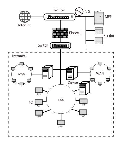
Connect the products to the outside of the Internet through a firewall as shown in *Figure-2: Correct product connection on network*.
