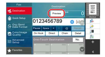
The machine starts scanning the original. When scanning is completed, the preview image appears on the panel.
