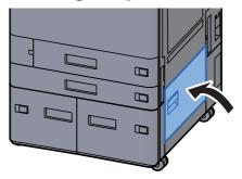
If the optional side feeder is installed, return the side feeder to the original position.
