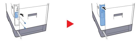
6 Insert the power cord into the socket and turn on the power switch.
