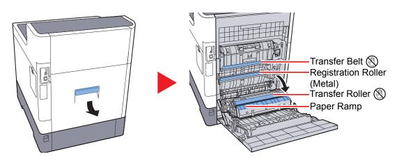
Wipe away the paper dust on the registration roller and the paper ramp using the cloth.
