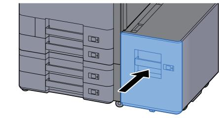
**4** Insert the indication on the sheet so as to match the size and type of paper to be placed.
