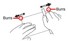
Before loading Hagaki (Cardstock), fan them and align the edges. Hagaki (Cardstock) should be fed from the multipurpose tray with the print-side down or the cassette and the optional paper feeder with the print-side up. If the Hagaki (Cardstock) paper is curled, straighten it before loading. Printing onto curled Hagaki (Cardstock) may cause jams.
