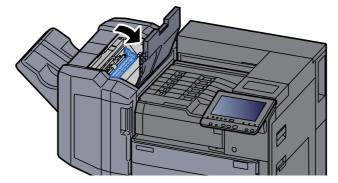
Open the finisher front cover. 5 Ø Open the conveyor guide (D1). 6 ß D1 Remove any jammed paper. 7 ß
