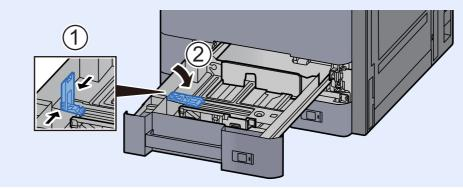
**3** Adjust the position of the paper width guides located on the left and right sides of the cassette.
