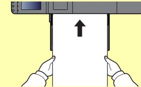
• After printing starts, catch the paper when it is output so that it does not fall. When using the main tray as the output location, do not stand up the stopper.
