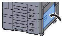
**5** If the optional side feeder is installed, return the side feeder to the original position.
