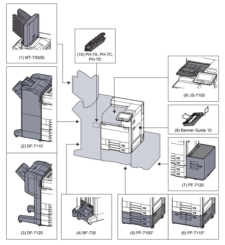
\* If the following option is installed, toppling prevention kit must be installed: PF-7100, PF-7110
